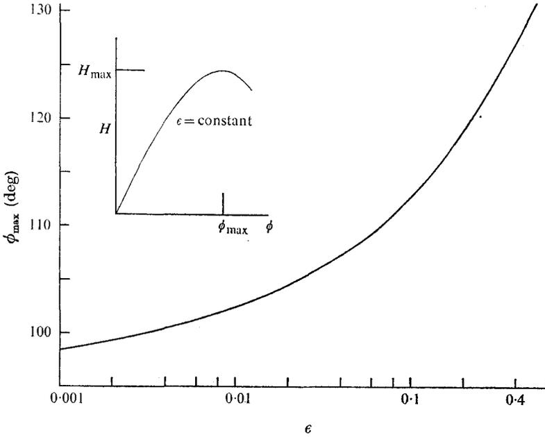
FIGURE 4. The maximum attainable angle  $\phi_{\max}$  versus the perturbation parameter  $\epsilon$ , which represents  $(\rho g r_0^2/\sigma)^{\frac{1}{2}}$ ; this result pertains to the situation sketched in figure 2, where the meniscus is attached to the end of the cylinder.
