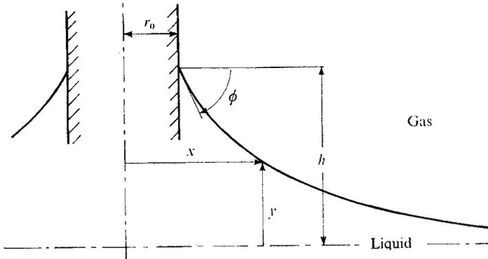
FIGURE 1. Definition sketch for a meniscus attached to the outside of a circular cylinder;  $0 \leq \phi \leq \frac{1}{2}\pi$ .
