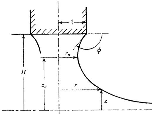
FIGURE 2. Definition sketch for the case  $\phi > \frac{1}{2}\pi$ , when the meniscus is attached to the bottom of the cylinder.
